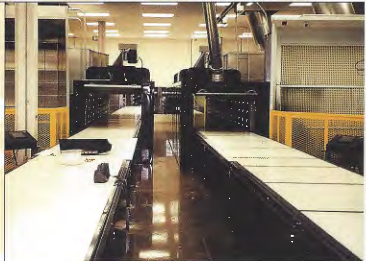
High velocity air convection ovens with butyl belt slider bed conveyors
