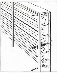
The modular design of Blasdel Enterprises, Inc. infrared ovens make them an excellent capital investment. Simply by changing the framing and configuration, the same infrared units may be used for many applications throughout your facility. Occasionally, increasing the wattage of the element may be necessary to meet new process specifications. Higher wattage elements will fit in the same housing, however, some control panel modifications may be required.
