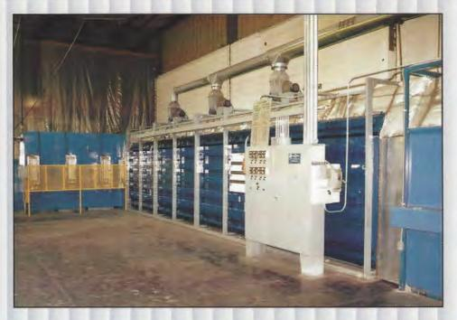
Using infrared to cure powder coatings is an excellent way to obtain a fast cure on a variety of parts. A gel state is reached quickly, usually within one to two minutes, on most parts. Total cure is possible in as little as two minutes. For applications with an existing convection oven, an infrared booster oven may provide the temperature increase required when converting a liquid system to powder.
