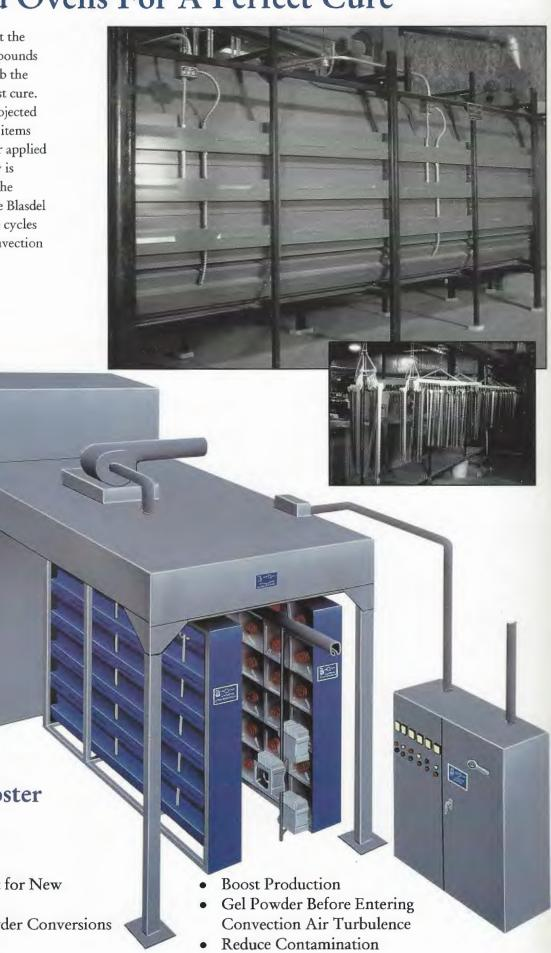
Blasdel Infrared Booster For Existing Convection Oven
