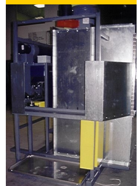
FINISHING CELL SYSTEM WITH VERTICAL OVEN CONTAINING C-O-R ELEMENTS, SPRAY BOOTH AND SPINDLE CONVEYOR
